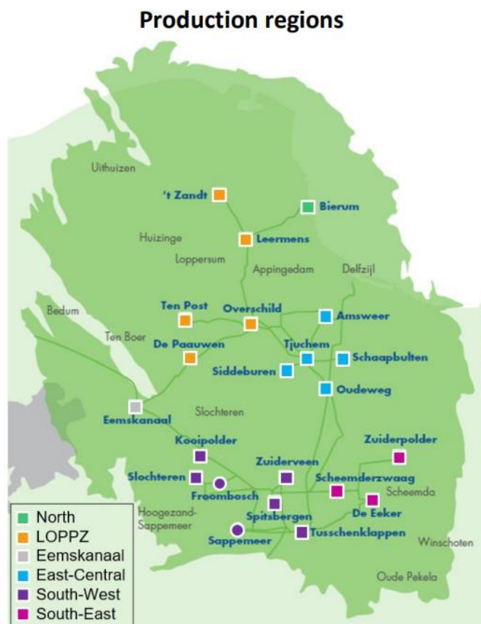
Figure 9 Overview of gas well clusters and past production regions in the Groningen field. Source: NAM (2020). The status of wells in these clusters is summarized in Table 1.
